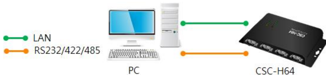
Figure 2-8 connection between CSC-H64 and a PC
