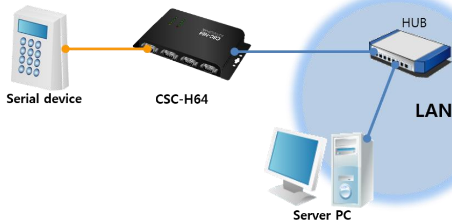
Figure 1-3 applied to LAN
