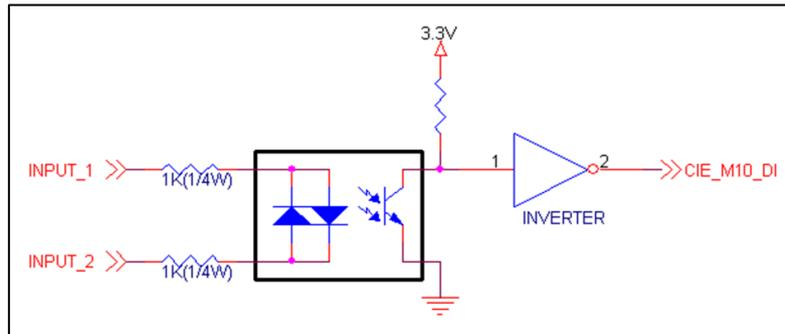
Figure 1-8 a circuit of the input port
