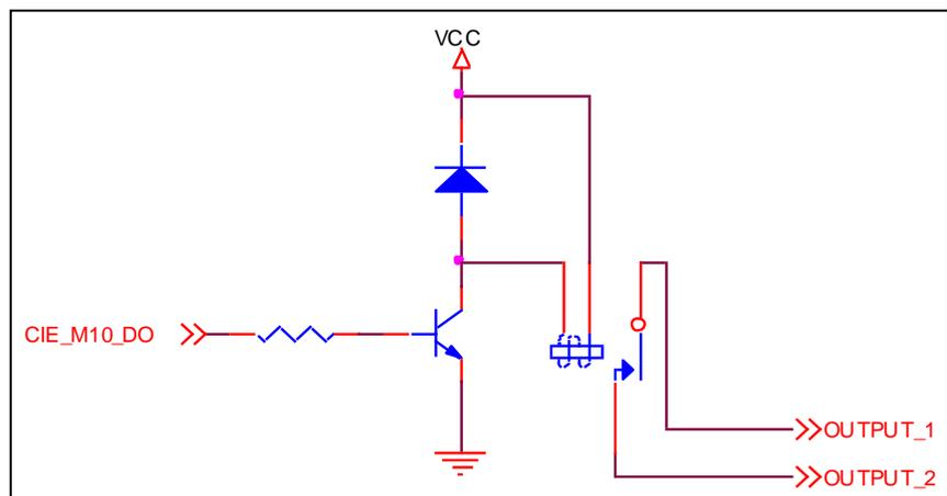
Figure 1-10 a circuit of the output port
