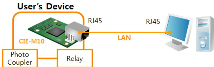
Figure 2-1 the connection between CIE-M10 and a PC
