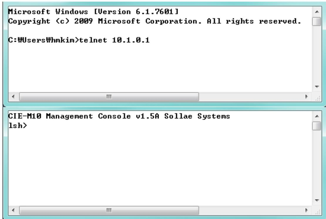
Figure 7-6 log in to CIE-M10 on TELNET
