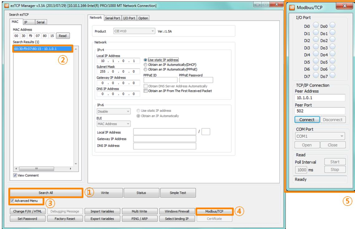
Figure 2-3 Modbus/TCP test program of the ezManager
