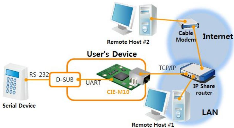
Figure 1-5 serial device server
