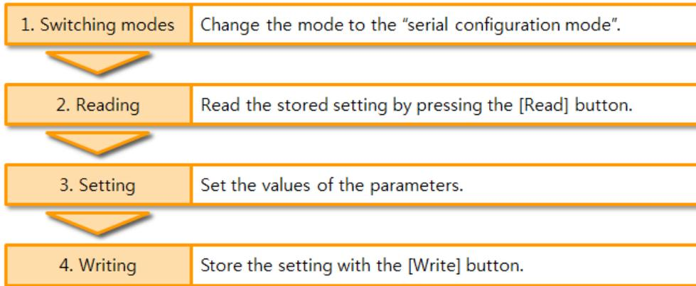
Figure 3-3 procedures for configuration via serial port
