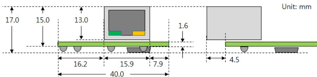
Figure 1-7 Front and Side view
